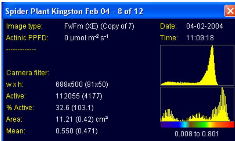
The imager software calculates a new average value for the selected area and displays this along with the value for the original entire image in the Image Information display box. The physical areas of the original and selected portion of the image are also displayed.
