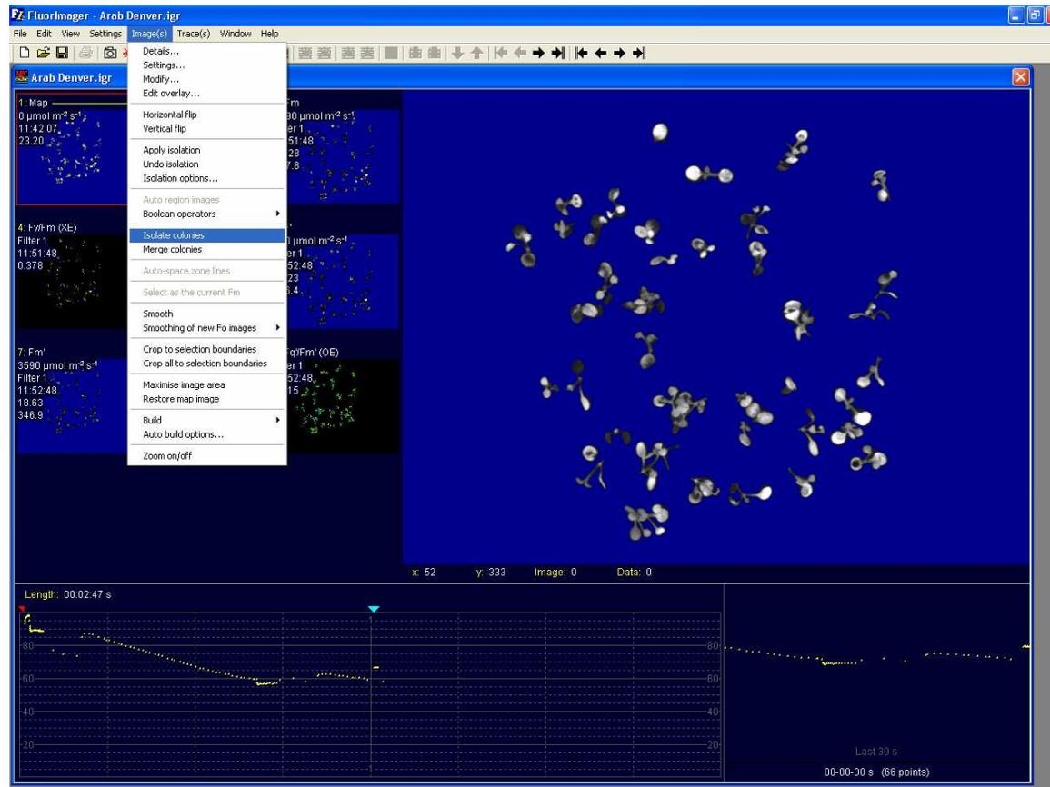
If necessary, Image Modification tools can be used to separate plants that overlap. Also a MERGE COLONIES command allows several colonies to be grouped as one sample if this is required.
