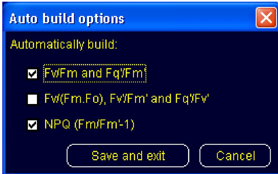
During the experiment, data are used to construct images within 1 second of the data being collected. Thumbnail images ( $F_o$ ,  $F_m$ ,  $F'$  and  $F_m'$ ) appear on screen as the experiment progresses. The user has the option of displaying up to 6 different parameter images based on these values. The selection is made under Auto Build Options in the Image(s) menu.
