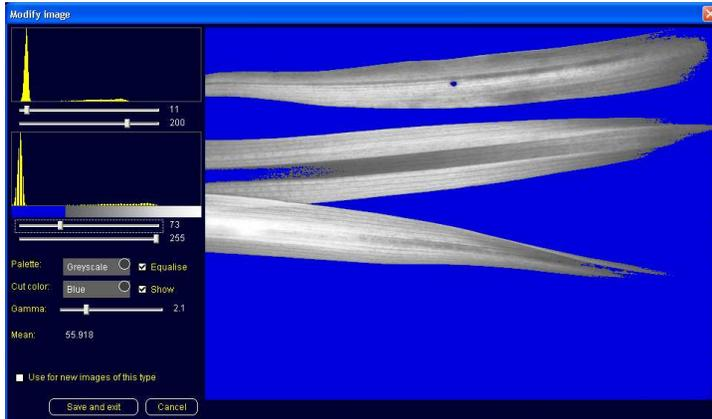
Too many pixels have been deactivated in the middle image. Areas of the leaf have been cut, especially those where variegation has resulted in low signals.
