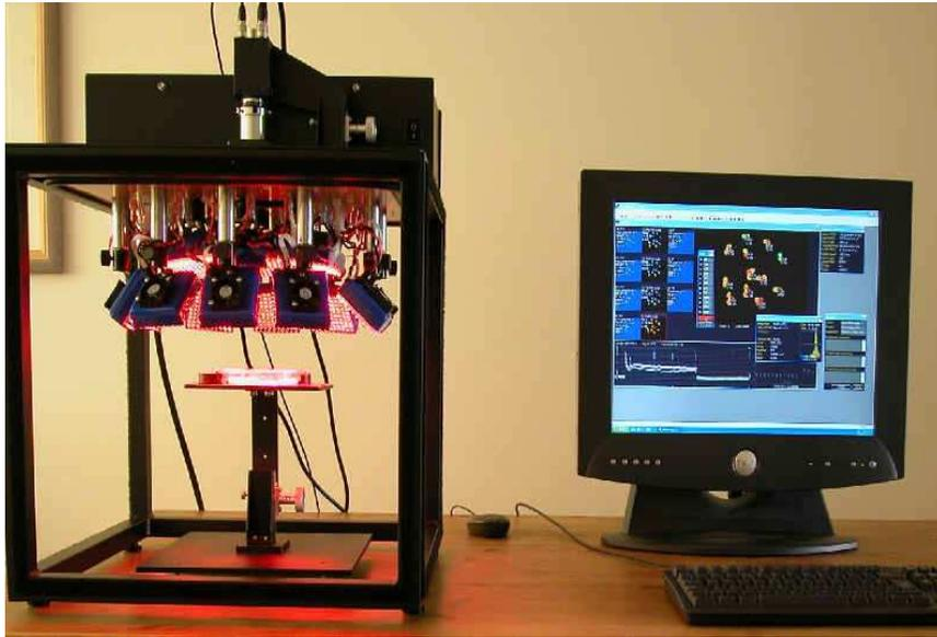
The **cflmager** is built around an array of 1600 LEDs configured in 16 blocks. This arrangement provides even incident irradiance across a 10 x 12 cm standard area.
