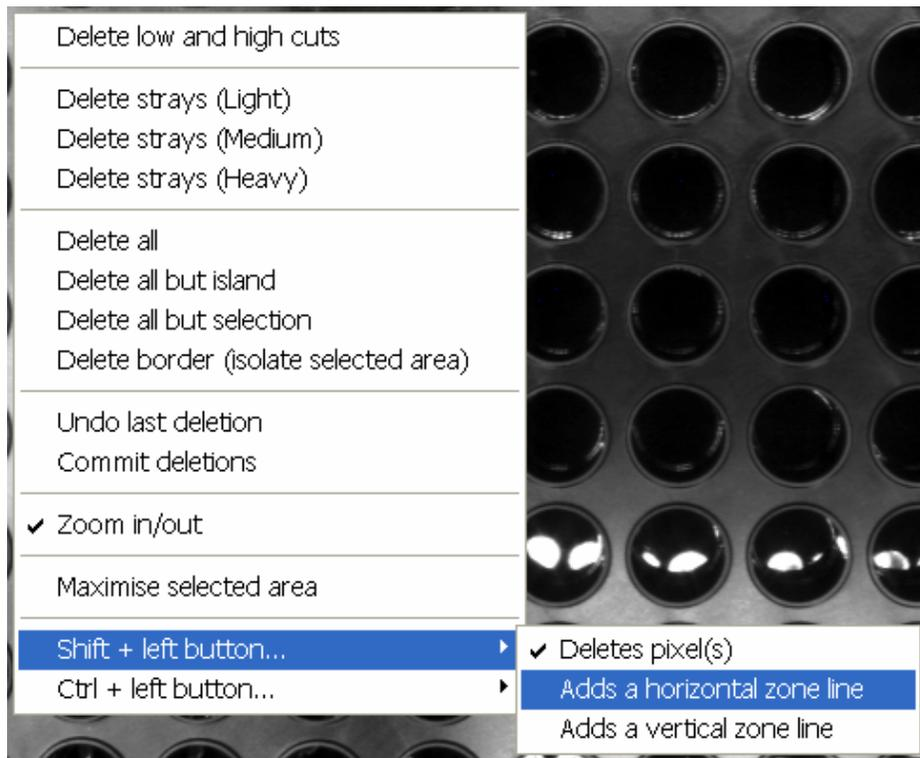
**Zone lines are added and deleted using mouse clicks. Line positions selected using a reflected light image of an empty plate can be copied and pasted onto the image of a plate containing samples. In this way the sample plate does not need to be exposed to light before the experiment, and dark adaptation is not disturbed.**
