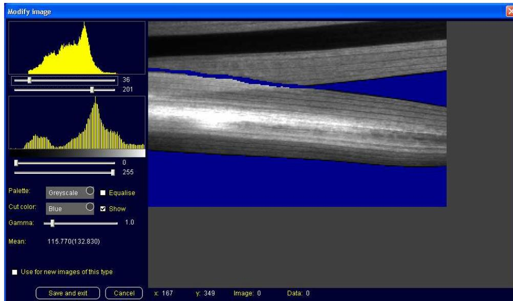
Here, the zoom function has been used to zoom in on the area where the two lower leaves overlap, a line of pixels has been cut to separate the leaves. The Auto Region Images command may now be used to identify the three leaves as individuals as shown on the next slide.
