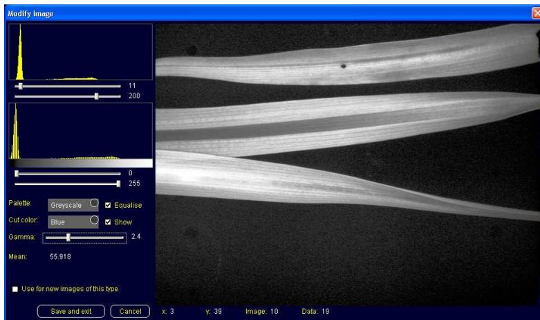
The initial map image (left upper) may be modified by several image manipulation tools within the imager program. The simplest way to isolate pixels that make up the images of the leaves is to click on Apply Isolation within the Image(s) menu. This deactivates pixels with low fluorescence values, clearly defining the leaves (left lower).
