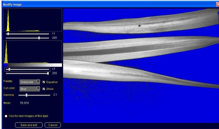
Active pixels are shown in grey scale. Inactive areas are shaded blue. A slider is used to activate and deactivate pixels.
