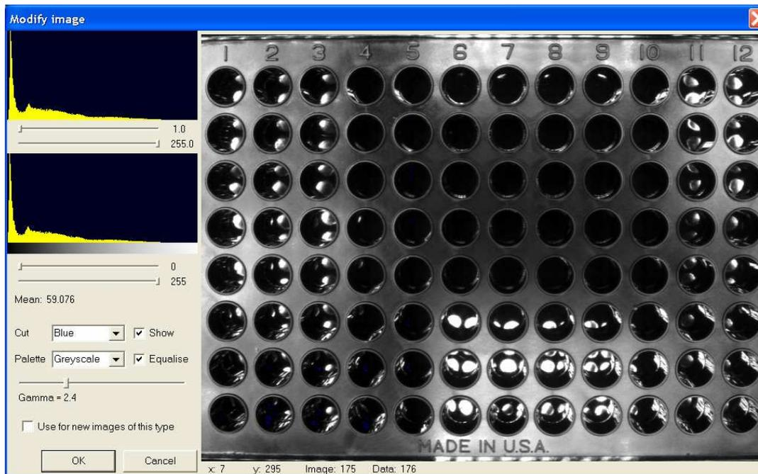
A 96 well plate is useful for growing small plants such as *Arabidopsis* for screening. The Imager software can calculate fluorescence values for all 96 plants simultaneously.
