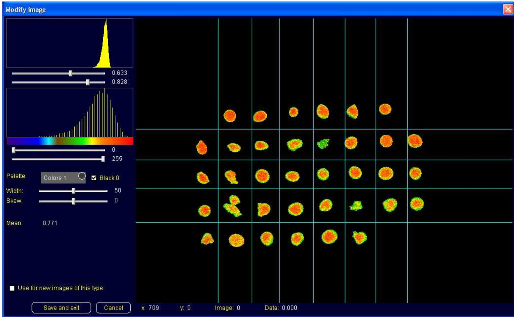
Values for sample area and for the imaged data (from the previous slide) have been copied to the Clipboard and pasted into Excel. The Excel data has an array corresponding to that of the zone data. Zero values indicate empty zones in the array.
